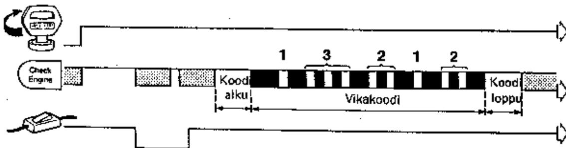
Fault code on the picture is "13212", which is, according the fault list, means that Throttle position potentiometer signal on full load is too weak.
