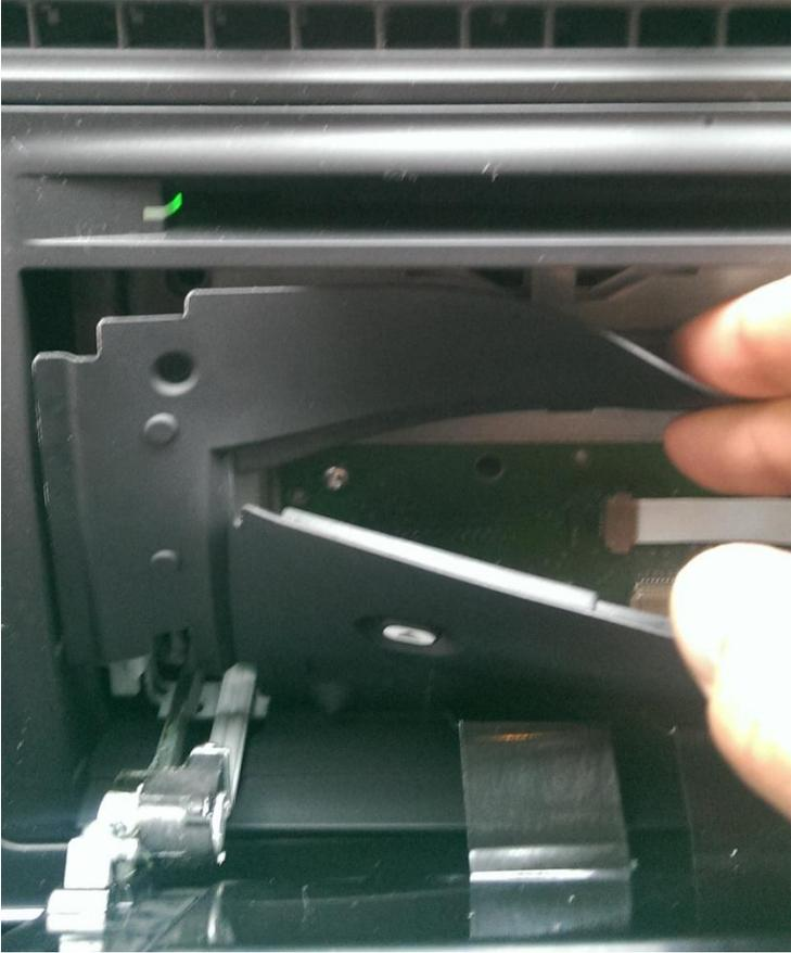
Use a cotton swap with (and/or without) alcohol and an extension, like a straw as shown. (see also example last page) With this extension you can reach the laser which you should be able to see right of the centre . (appr. 2 cm right from the middle of the unit and some 8 cm penetrated inward)
