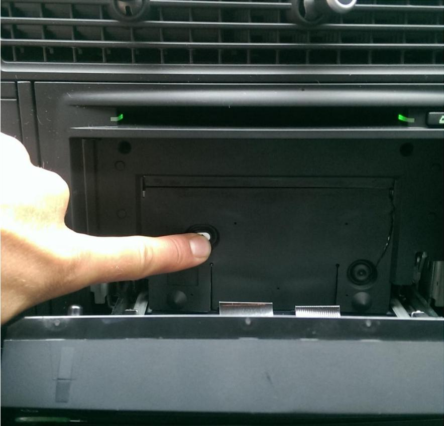
Pict. 3 Carefully remove the rubber flapper in front of the unit (it has sticky tape)
